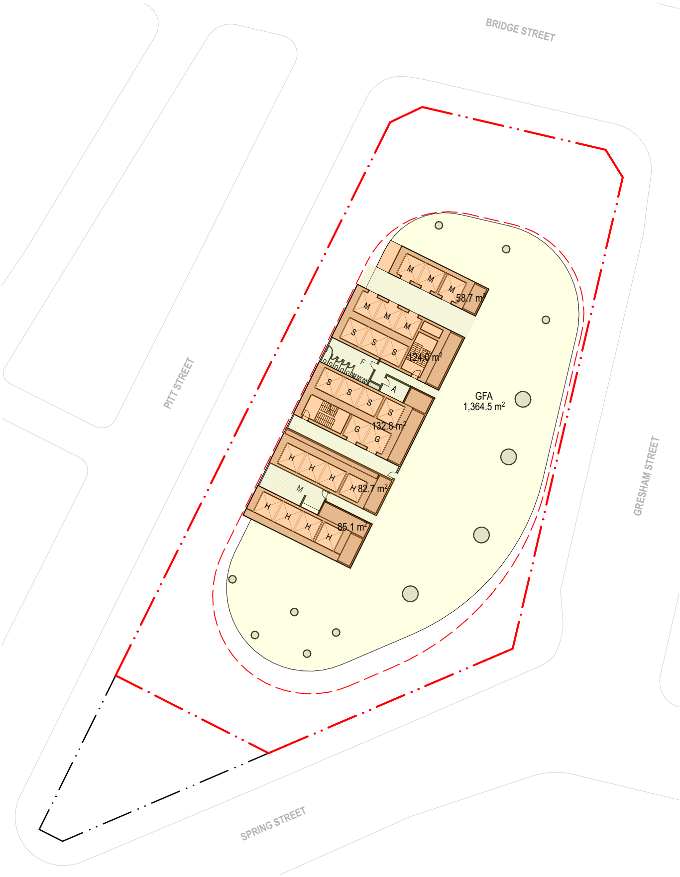
Mid Rise Commercial Floor Plan GBA = 1849.3 m2 GFA = 1698 m2 Core = 483.3 m2 Core 483.3 / GBA 1849.3 = 26.13%
